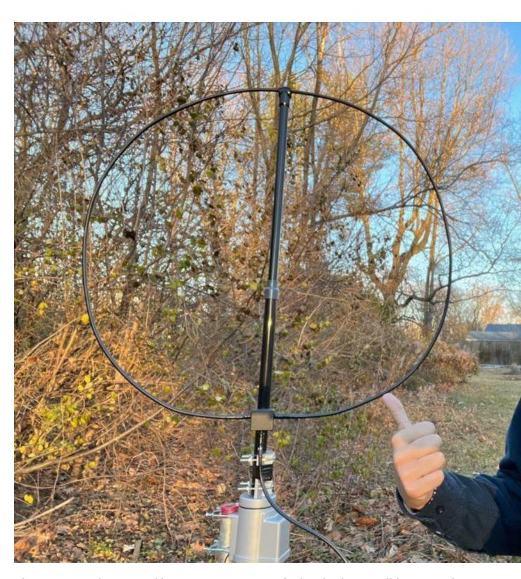
I have a magnetic loop on an old TV antenna rotator in my backyard. It has a small footprint and has helped me pull in AM stations from California to Colombia from here in central Illinois.
